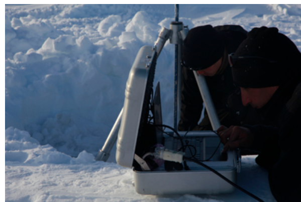
NPS students from left to right, Lt. George Suh and Lt. Brandon Schmidt scan an ice keel using sonar during their ten-day research trip to the Arctic. The trip, sponsored by the Office of Naval Research, was part of the Navy's Ice Exercise 2011.
