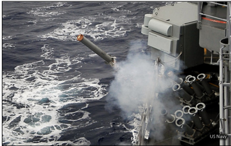
Figure 24: Lockheed Martin’s ALEX system (From Lockheed Martin 2012)
