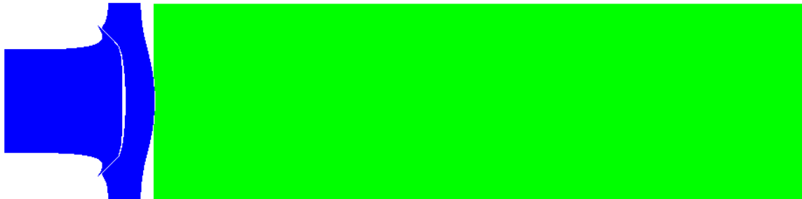
Figure 57: Visualization of the deformation effect due to the presence of an air gap between barrier and acceptor charge.
