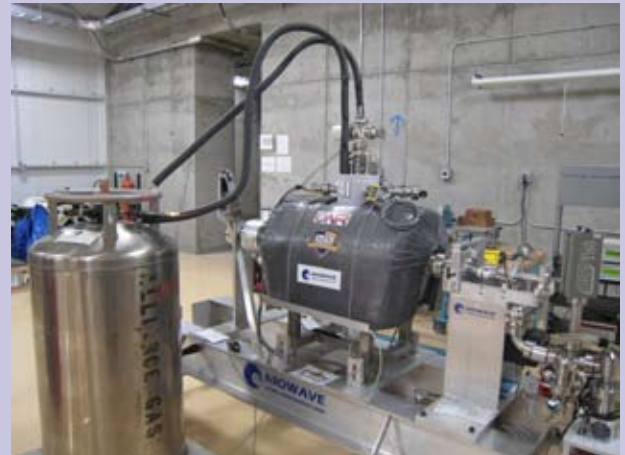
Mark I (center) connected to a liquid nitrogen tank (left) in the Beam Physics Laboratory
