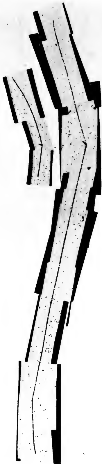
Disintegration of boron by fast neutrons
