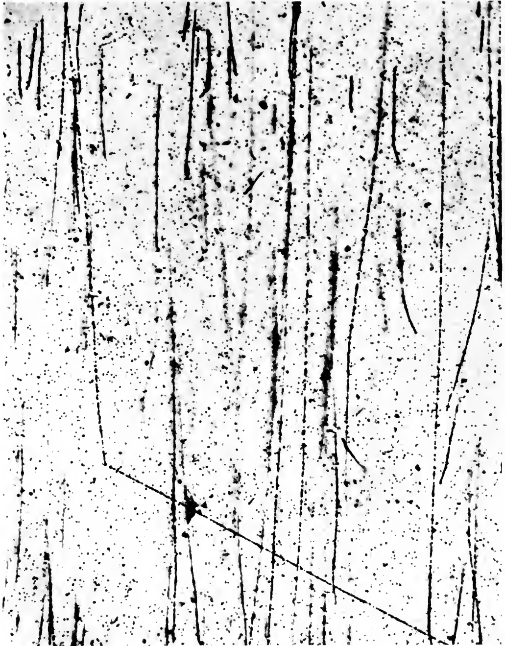
Tracks of protons and \alpha -particles
