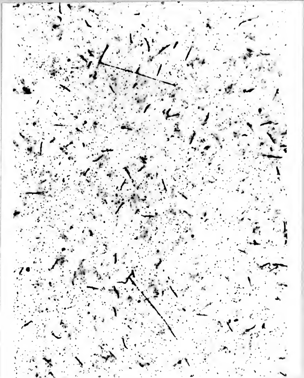
Tracks from the disintegration of lithium and boron by slow neutrons
