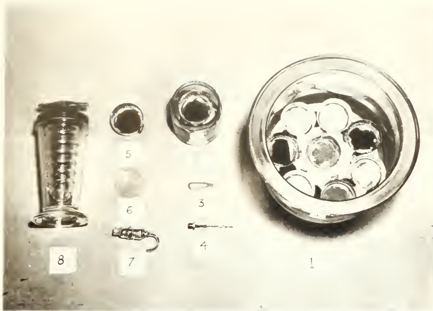
Fig. 1. Equipment Used During the Project 1. Desiccator, 2. Jar, 3. Weighing Funnel, 4. Squib, 5. Aluminum Cup, 6. Watch Glass, 7. U Tube, 8. Gas Washing Bottle
