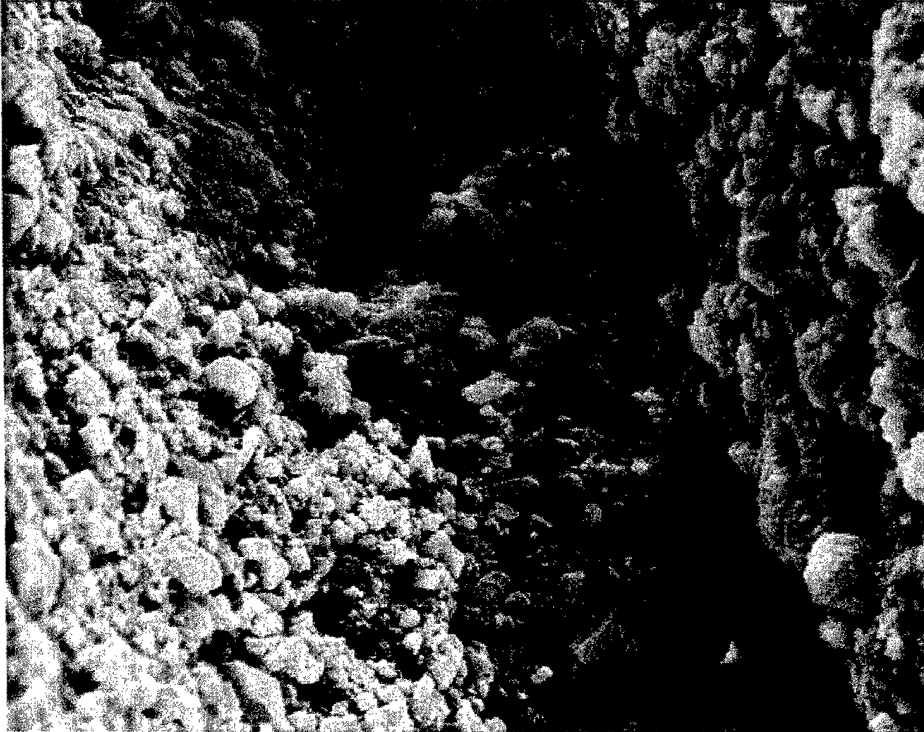
Figure 6-19 – Ewa 30 Day cemented sand at 2000x magnification.
