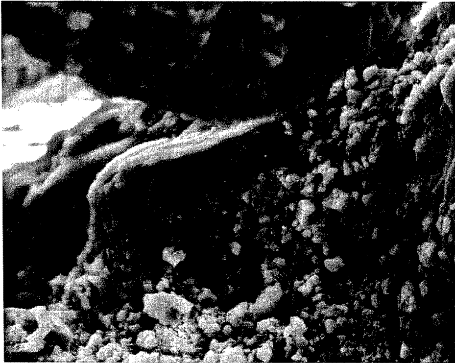
Figure 6.14 – Ewa unaged sand at 1000x magnification.
