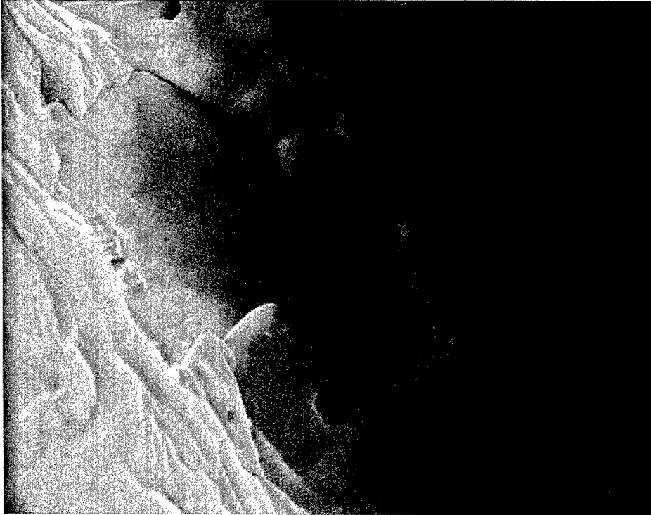
Figure 6.11 – Waikiki 60-Day cemented sand at 2000x magnification.
