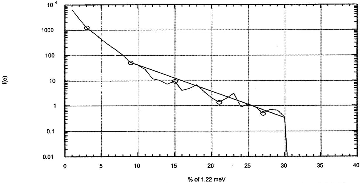
**Figures 17 and 18. Energy and Electron Distribution plots with Ti/Te=0.25. Note the lower electron temperature (compared to Case1) as a result of ion fluctuations (straight line on distribution plot depicts energy range to determine temperature).**
