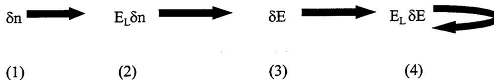
**Figure 2. Plasma instability feedback loop for Raman backscatter growing from noise.**
