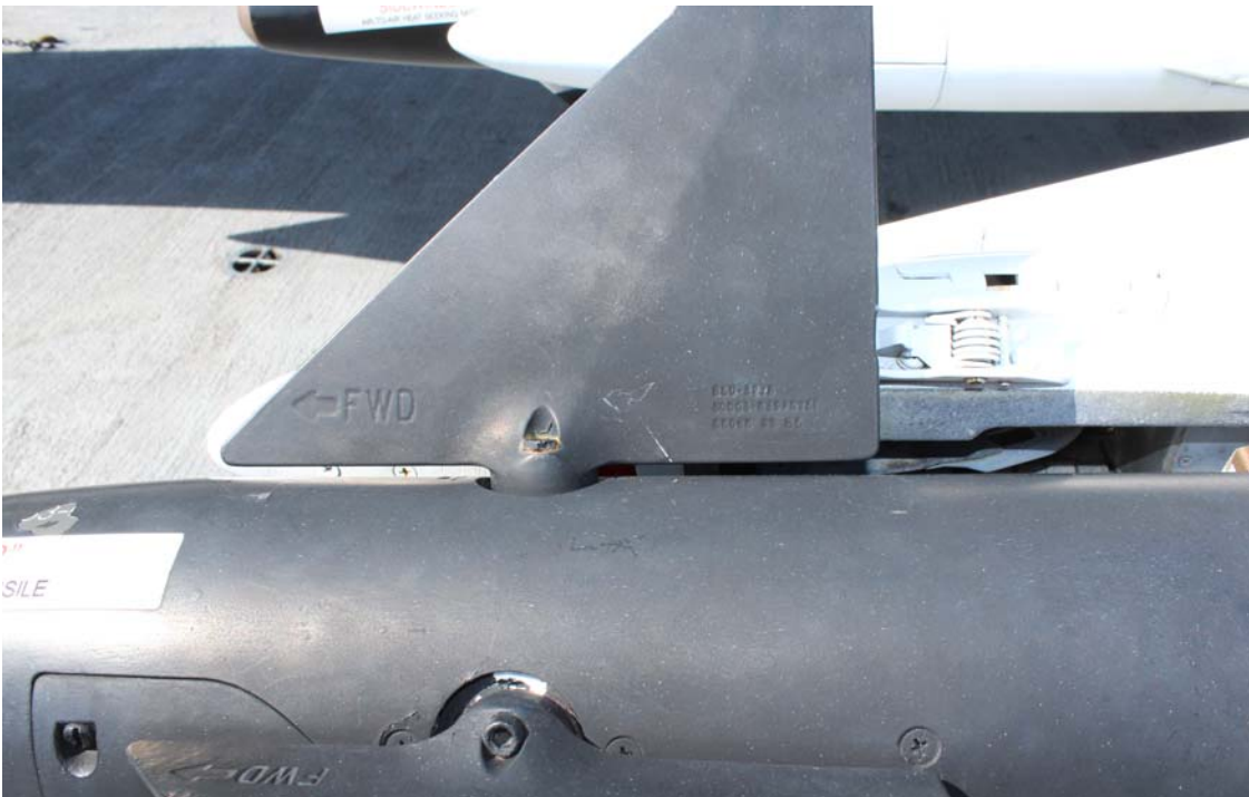
Figure 4. Picture depicting protruding bolts holding canard to hinge.
