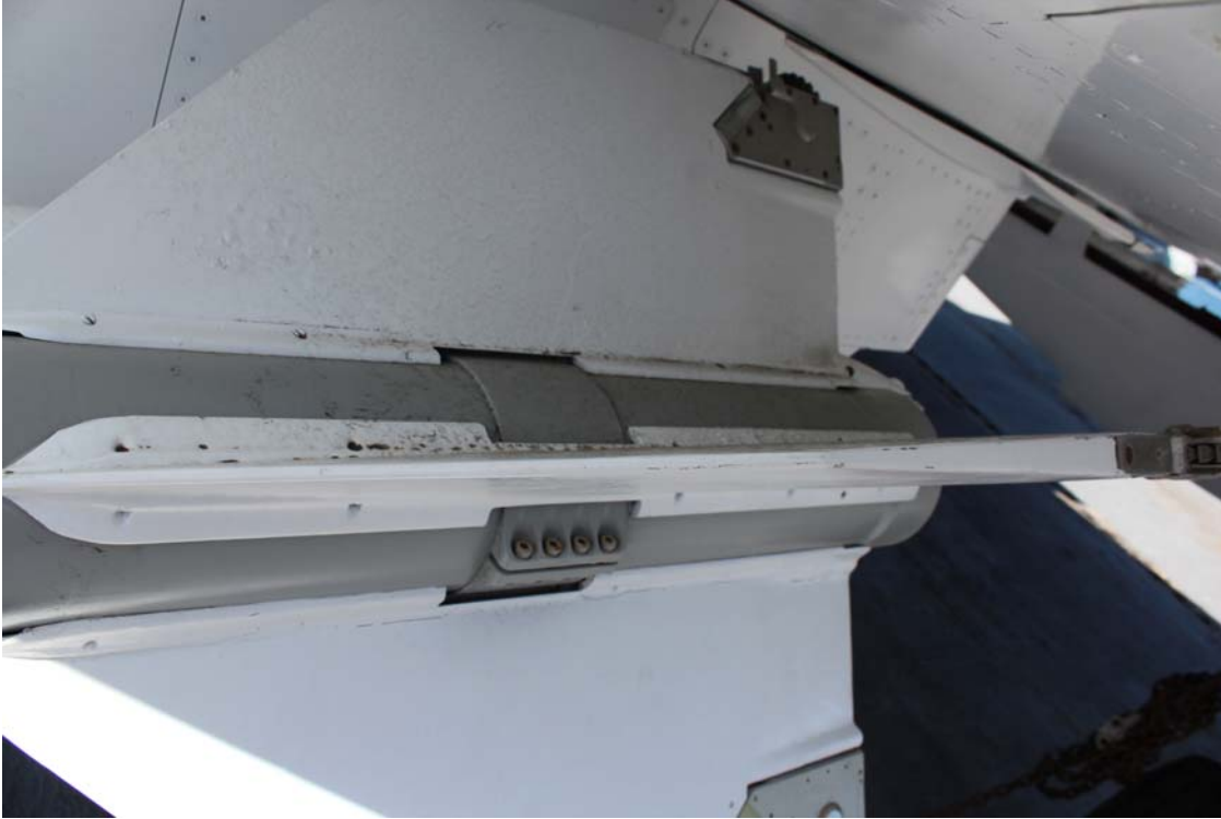
Figure 5. Picture depicting the method of attachment of tail fins to fuselage.
