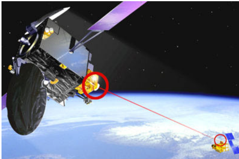
Figure 2. Artemis and SPOT 4 Communicating via the SILEX system – Artist's Impression (From: [Oppenhäuser 2001])
