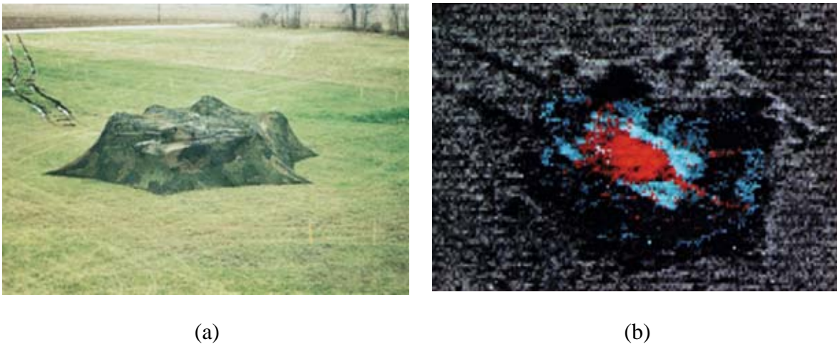
Figure 9. (a) Visible-light photograph of tank under canopy, (b) Lidar image of tank with camouflage net gated out (From: Gschwendtner & Keicher, 2000)
