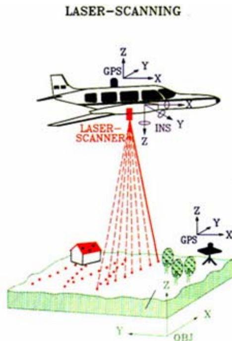
Figure 2. Lidar system integration (From: Spencer B. gross, inc. 2007)
