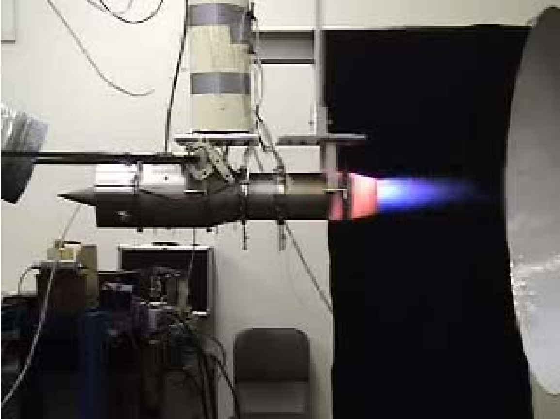
Figure 21. Turbo-Ramjet at Maximum Afterburner at M_\infty = 0.15
