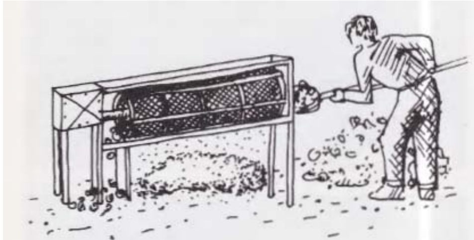
Figure 20. Sieving devices remove unwanted particles of organic matter or larger rocks. Sieves range from simple screens to hand-cranked or motor-driven mesh drums. Drawing from Earth Construction Handbook by Gernot Minke, page 42.
