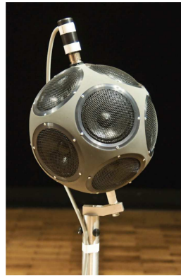
(b) Tilted dodecahedron loudspeaker mounted for room acoustic measurements [Kun11]
