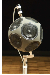
(b) Loudspeaker array used for the synthesis
