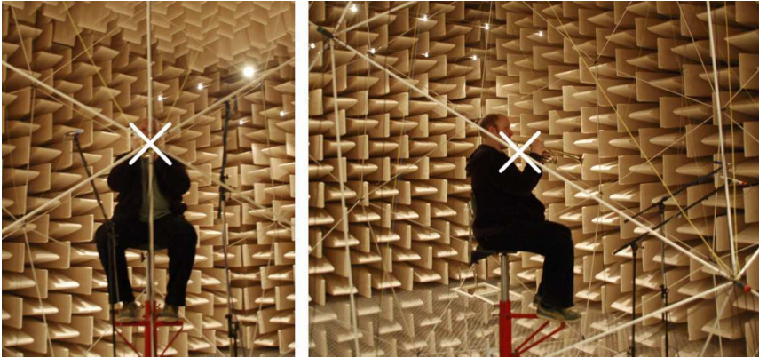
Figure 3.13.: Measurement of trumpet directivity in the surrounding spherical microphone array. Approximative center of microphone array marked with a white cross [BH11; Pol12e].
