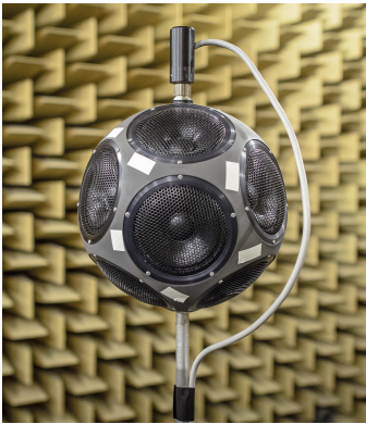
(a) Dodecahedron loudspeaker mounted for directivity measurements
