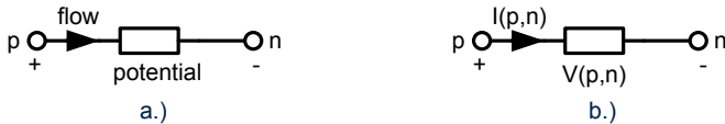
Figure 3.5: Associated branch, potential and flow in VERILOG-A according to [FM98]. a.) Abstract representation. b.) Electrical voltage and current reference direction for a branch.
