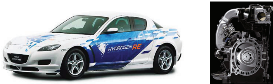
Figure 8: MAZDA RX-8 Hydrogen RE vehicle and the H 2 rotary engine [8].
