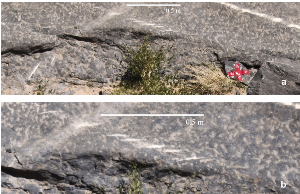
Fig. 21: Both pictures have the same pixel dimensions and were shot from spot 1. Picture a is shot with a focal length of 200 mm, whereas picture b is shot with 400 mm. The resolution is clearly higher with 400 mm, although the effective resolution was digitally reduced during the rendering process of Autopano Giga.
