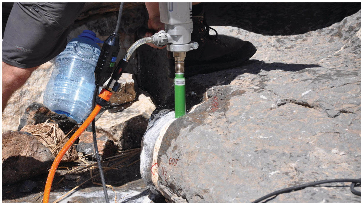
Fig. 15: Drilling plugs out of vein set 1 using a CARAT hands-free core drilling machine type 2011.
