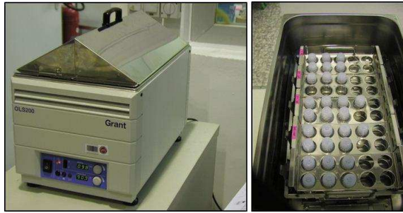
Figure 22: Shaking oil bath at 90 °C used for aqueous durability tests. Closed (left) and open (right).
