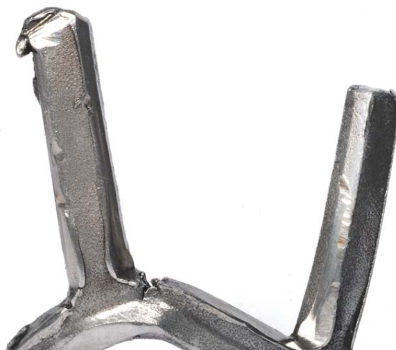
Figure 1-1: Damaged cages in a tapered roller bearing in high-speed trains
