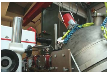
Figure 1. OU's AALGG. The Ultra 8 camera was mounted to image inside the chamber, via a small mirror.
