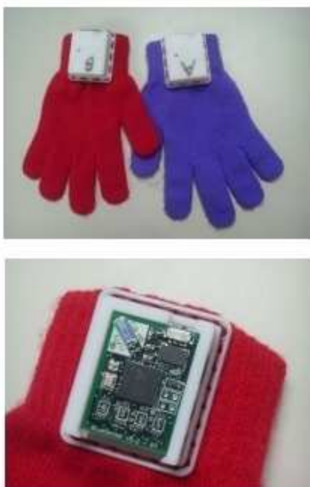
Figure 3: Gloves with accelerometer (top). Close up of wrist-mounted accelerometers (bottom).
