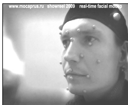
Figure 4: Demonstrator with glued on the face reflectors
