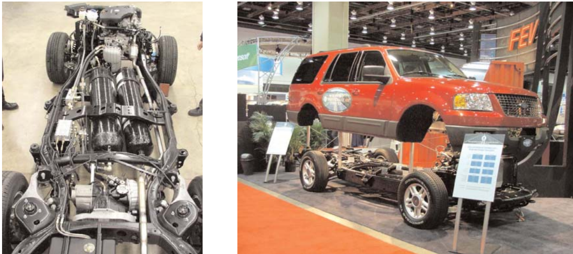
Figure 2.8: A complete view of full hydraulic hybrid SUV at SAE Congress [52]
