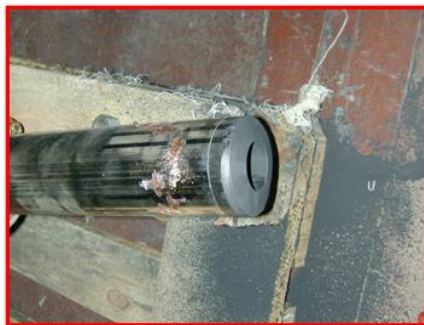
Fix contact of Pole B manipulated to damage
