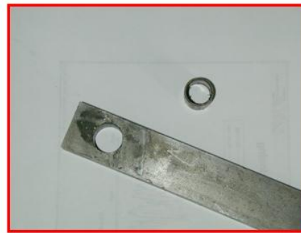
Remove bush of connecting rod of Pole A
