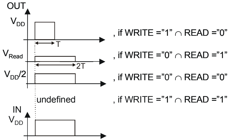
Fig. 9.3 Wordline driver conditions for a read/write/protect.
