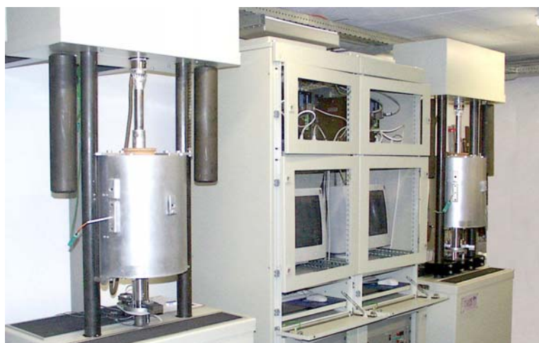
Fig. 5-10 Creep testing machine at LFW.
