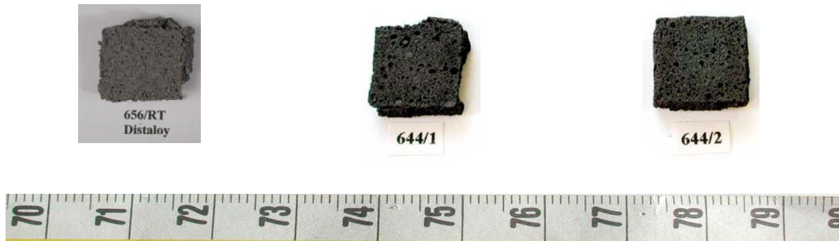
Fig. 6-17 Stereoscopic macrographs of Distaloy foams having different densities, tested at RT (left), 450°C (middle) and 600°C (right), respectively.
