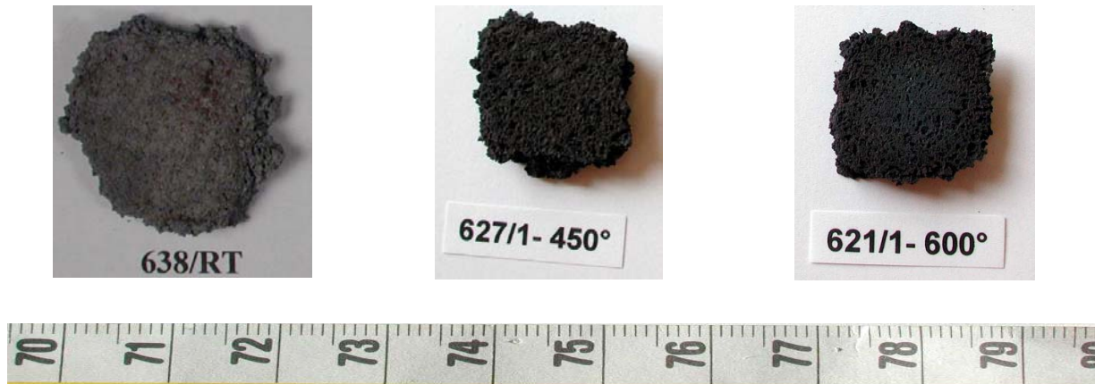
Fig. 6-27 Stereoscopic macrographs of Astaloy foams having different densities, tested at RT (left), 450°C (middle) as well as 600°C (right), respectively.
