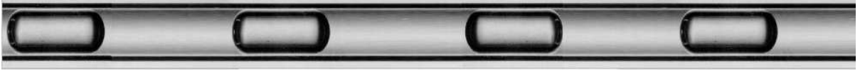
Figure 1.1: Bubble-train flow consisting of air bubbles in water flowing through a 1.2 mm glass capillary. The capillary is submerged in water to reduce refraction.
