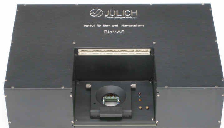
Figure 4.7: Photograph of the BioMAS headstage housing including a head in the lower position. The horseshoe-shaped headstage contains two PCI ports to allow an alternative connection of the head in a top position. Connection to the main amplifier is established by two parallel ports at the backside of the headstage.
