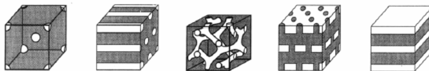
Fig 1. 1 Schematic representations of the ordered microstructures obtained for diblock copolymer melts; from left to right: body-centered cubic packed spheres, hexagonal-packed cylinders, gyroid, hexagonally perforated layers and lamellae. [14]
