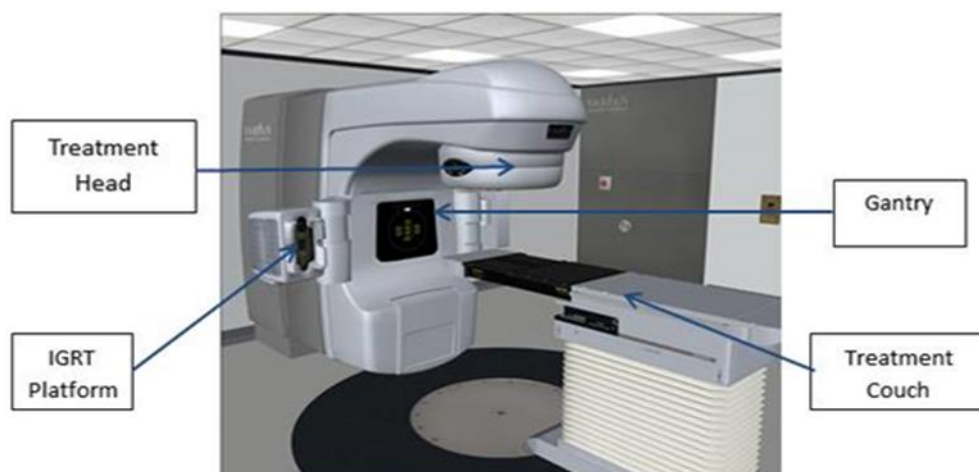
Figure 2.1: A Varian Clinac iX linear accelerator as modelled in VERT™ v 3.0. (Screenshot from UoP VERT™ platform with permission of Vertual Ltd, 2016)
