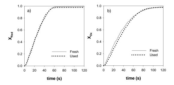
**Figure 5.** Conversion vs time curves for (a) reduction and (b) oxidation reactions for fresh and used particles. Reduction in  $N_2$  and oxidation in air at 1000 °C in TGA.
