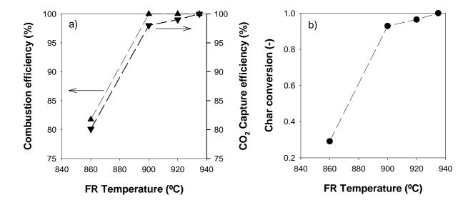
**Fig. 4.** (a) Combustion efficiency in the fuel reactor and CO<sub>2</sub> capture efficiency and (b) char conversion, as a function of the fuel reactor temperature
