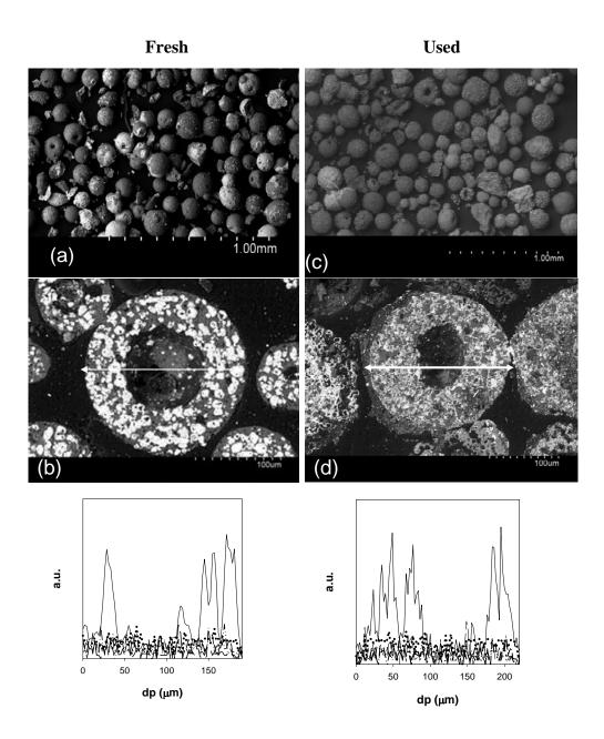
**Figure 6.** SEM images of fresh (right) and used (left) particles after 10 h in CLOU unit: (a, c) image of the particles; (b, d) image and EDX line profile of Cu (—), Ca (---), K (----), P (---), and Na (···) in a cross section of a particle.
