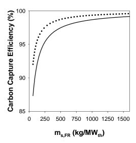
**Fig. 8.** Carbon capture efficiency as a function of the fuel reactor inventory for biomass at two different temperatures in the fuel reactor:  $900^{\circ}\text{C}(--)$ ,  $920^{\circ}\text{C}(---)$ .  $\eta_{\text{CSS}}=0$ ;  $\phi=1.1$ .
