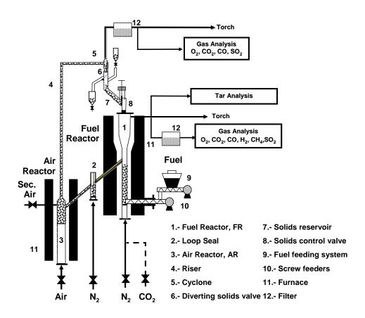
Fig. 2. Schematic view of the ICB-CSIC-s1 unit for the CLOU process  $(1.5 \text{ kW}_{th})$ .
