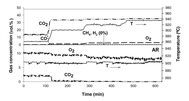
**Fig. 3.** Evolution of the gas composition in the air and fuel reactors as temperature in the fuel reactor was varied.  $\dot{m}_{SF} = 0.24 \, kg \, / h$ .
