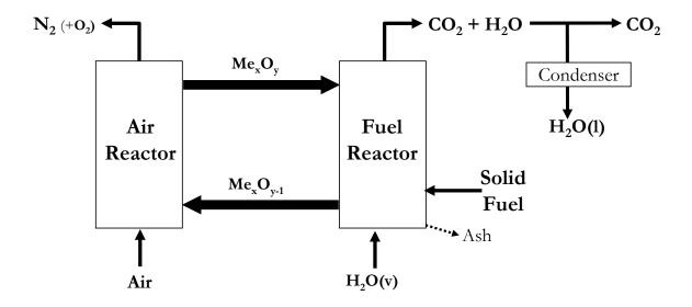
Fig. 1. Schematic layout of the CLOU system.
