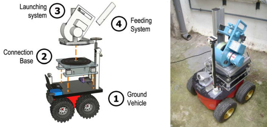
Figure 8: Deployment system components (left). (1) rover; (2) damping connection base; (3) launching system; (4) node feeder. Right: the implemented system.
