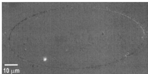
FIG. 2. Phase contrast optical micrograph of the area ablated by a single pulse at 22.6 \times F_m .
