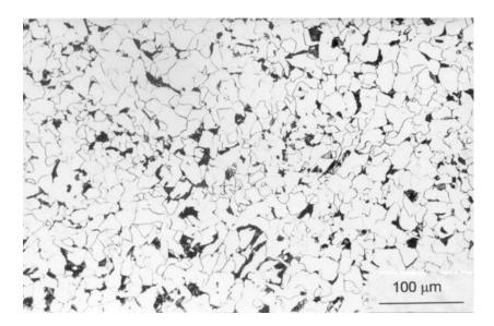
**Fig. 1.** (a) Dilatometric curve for given cooling and heating rates; (b) microstructure of ferrite and pearlite corresponding to dilatometric test.
