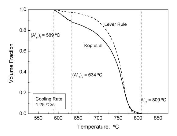
Fig. 11. Fraction curves obtained from lever-rule and Kop et al. method at given cooling rate.
