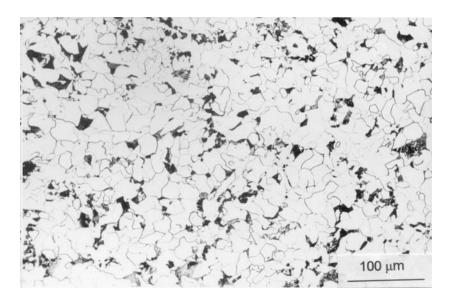
**Fig. 2.** (a) Dilatometric curve for given cooling and heating rates; (b) microstructure of ferrite and pearlite corresponding to dilatometric test.
