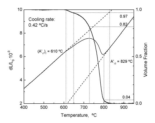
**Fig. 9.** Transformed austenite fraction calculated by lever-rule method at given cooling rate.
