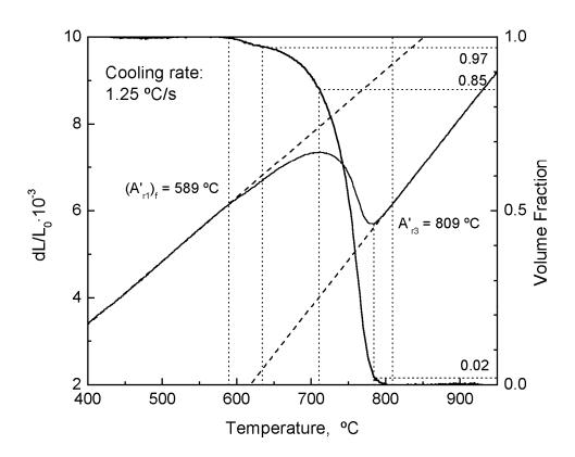
**Fig. 7.** Transformed austenite fraction calculated by lever-rule method at given cooling rate.
