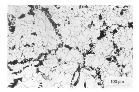
**Fig. 4.** (a) Dilatometric curve for given cooling and heating rates; (b) microstructure of ferrite and pearlite corresponding to dilatometric test.
