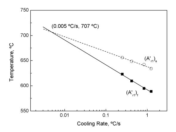
**Fig. 5.** Cooling Rate dependence of the initial  $((A'_{r1})_s)$  and final  $((A'_{r1})_f)$  eutectoid transformation temperatures, showing the intersection of regressions at 707 °C.
