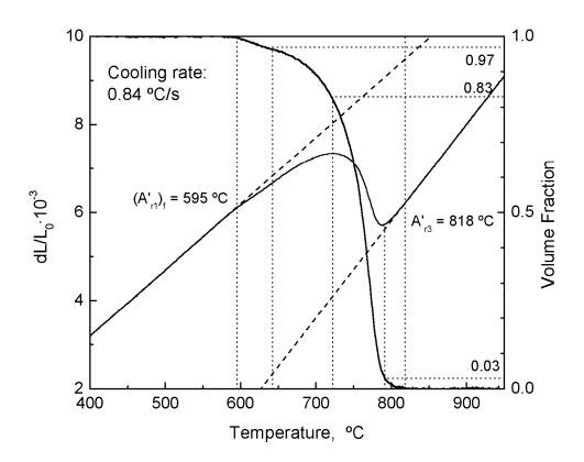
**Fig. 8.** Transformed austenite fraction calculated by lever-rule method at given cooling rate.
