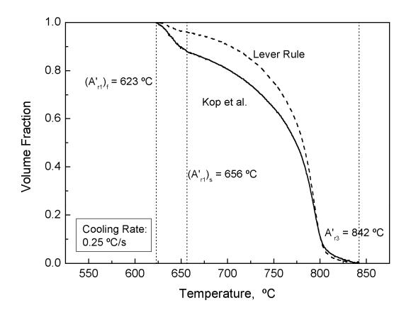
**Fig. 14.** Fraction curves obtained from lever-rule and Kop et al. method at given cooling rate.
