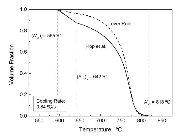
**Fig. 12.** Fraction curves obtained from lever-rule and Kop et al. method at given cooling rate.
