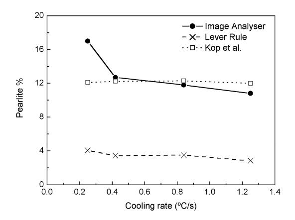
**Fig. 15.** Comparison of pearlite fraction calculated from both methods and the pearlite fraction measured by Image Analysis for the different cooling rates used.
