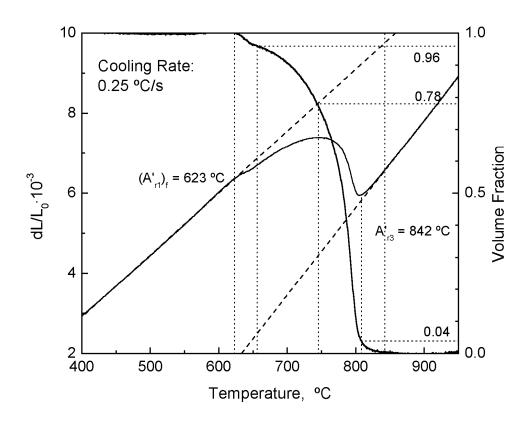
**Fig. 10.** Transformed austenite fraction calculated by lever-rule method at given cooling rate.
