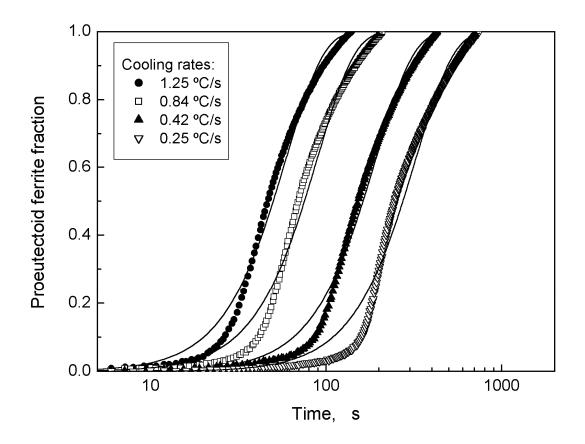
**Fig. 16.** Proeutectoid ferrite fraction calculated by Kop et al. method against time, for different cooling rates used (scatter graphs). The model for phase transformation kinetics based on Avrami's Law is also plotted (solid lines).
