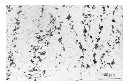
**Fig. 3.** (a) Dilatometric curve for given cooling and heating rates; (b) microstructure of ferrite and pearlite corresponding to dilatometric test.
