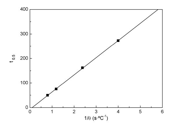
**Fig. 17.** Parameter  $t_{0.5}$  of transformation kinetics model against the inverse of cooling rate.
