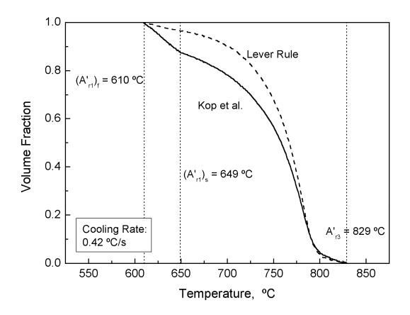
**Fig. 13.** Fraction curves obtained from lever-rule and Kop et al. method at given cooling rate.
