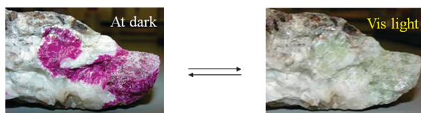
Fig. 2 Photochromic mineral (Hackmanite, \text{Na}_8\text{Al}_6\text{Si}_6\text{O}_{24}\text{Cl}_2 ) made by nature.
