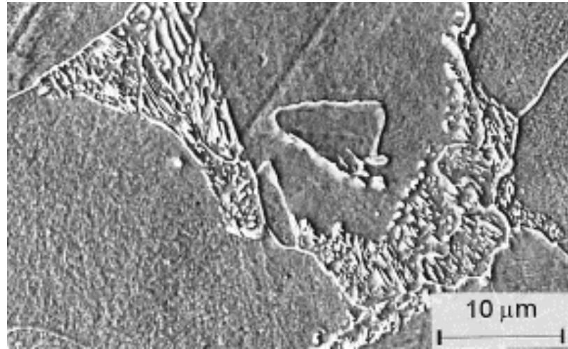
Figure 5. Microstructures obtained in the interrupted heating tests at 10°C below A_{c1} .
