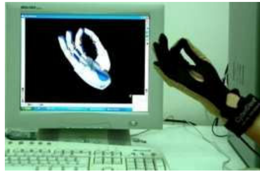
Fig. 2. Human hand with the sensorized glove connected to the mechanical hand simulator used in the data acquisition procedure.
