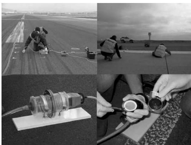
Fig. 2 Sampling of the PM 10 fraction of runway (02–20) dust.
