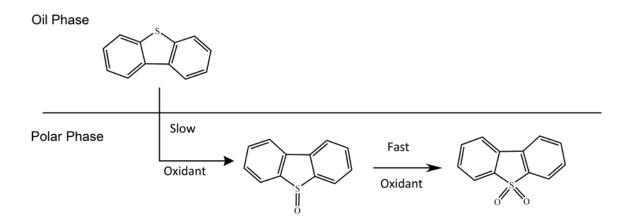
Scheme 2: The ideal reaction in ODS process for DBTs and BTs
