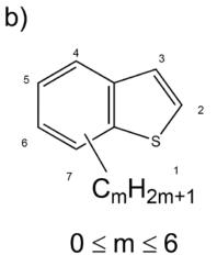
Scheme 1: Structure of DBTs (a), and BTs (b) present in light oils
