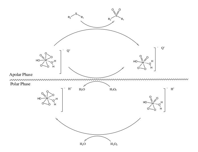
Scheme 4: Catalytic cycle of sulfur compounds oxidation.
