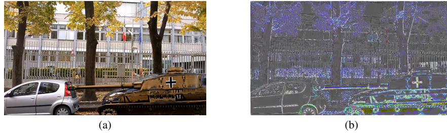
Fig. 1.7: Output of the Acutance filter on the edited tank video. (a) edited frame, (b) filter output. The image (b) stresses that the tank appears much more sharp than the rest of the image.
