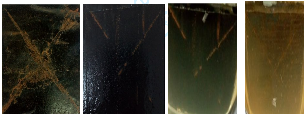
Figure 7: Image of coated steel after immersion in solution 3% (Wt/Wt) NaCl after 28 day paint) for coated sample by modified primer with PEA and by 30% modified PEA resin.
