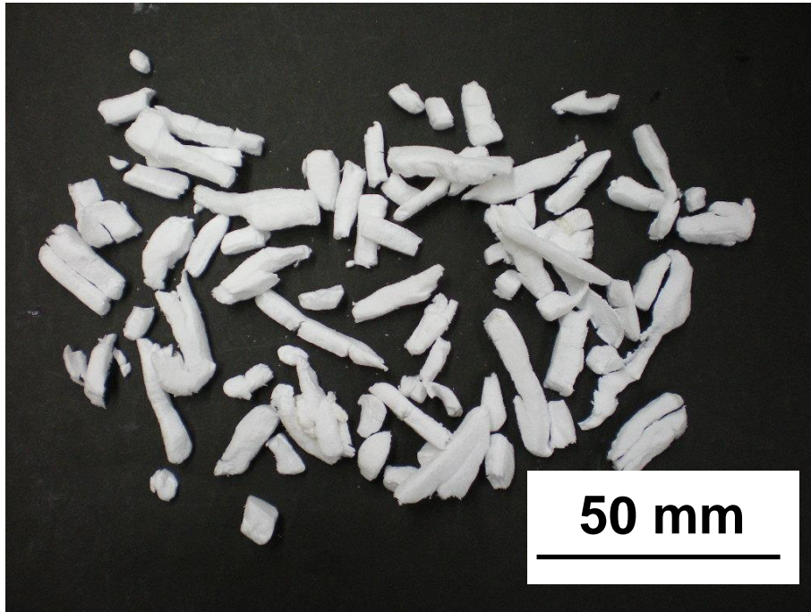
Figure 1. Aerogel prepared from cellulose nanofiber suspension frozen by liquid nitrogen from ambient temperature.
