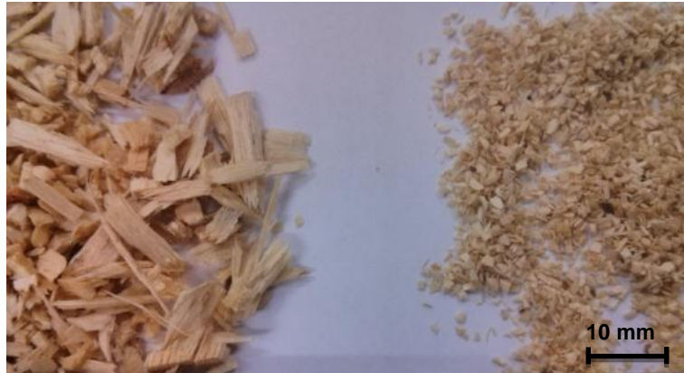
Figure 6: Wood chips 6 mm and smaller (left) and biomass knife-milled to under 2 mm (right)
