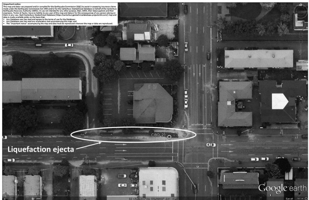
Figure 4. High resolution aerial photograph of Site 4: CPT-CBD-21 taken two days after the Christchurch earthquake illustrating “minor” liquefaction as defined in this study.
