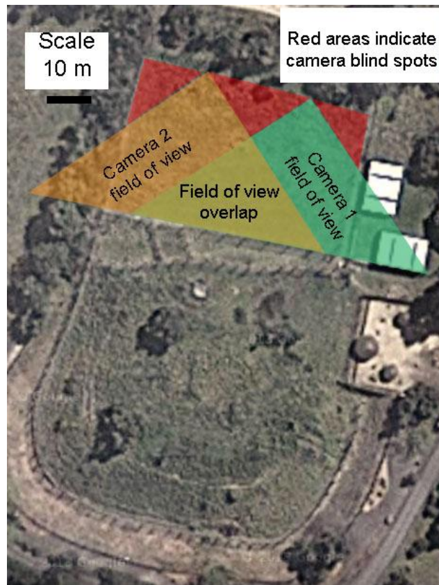
Figure 4.1. Fencecam layout. Red areas indicate camera blind spots, green indicates field of view for camera one, orange indicates field of view of camera two, yellow indicates overlapping field of view for both cameras.
