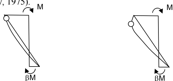
(a) Plastic Hinge at Member End (b) Plastic Hinge within Member Length
