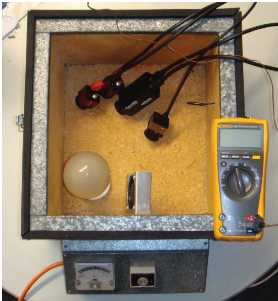
Figure 3: The temperature-controlled thermal chamber with the 4 cameras under test.
