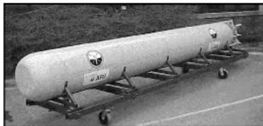
Fig. 3. The Seahorse AUV (Tangirala & Dzielski, 2007) Some of the advantages of a cylindrical hull are (Ross, 2006):
