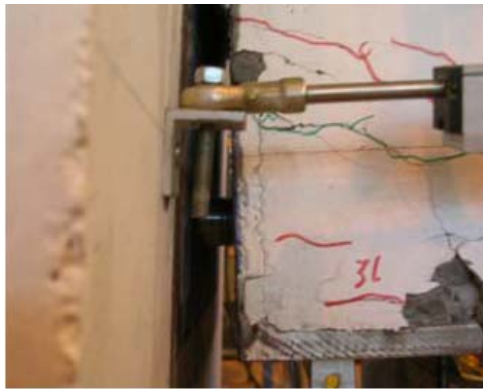
(a) Exposed shear key
