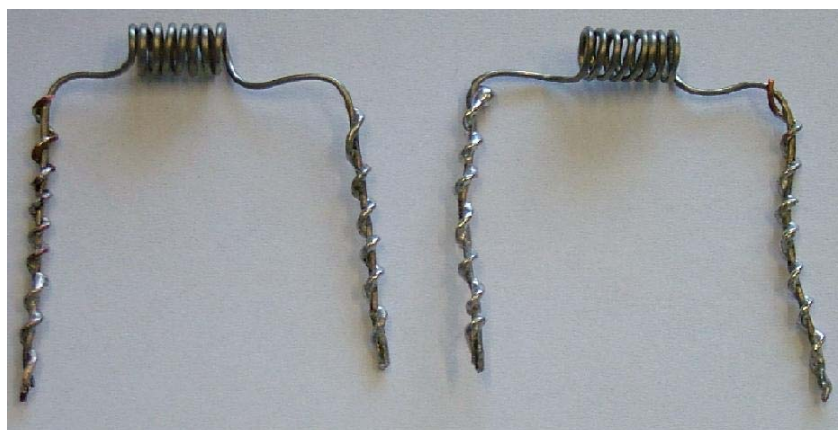
Figure 5.6: Hand made nichrome wire infrared filaments.
