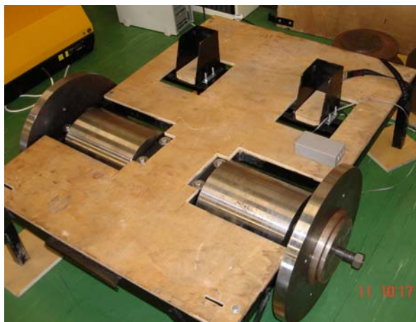
Figure 4.1 The wheelchair Dynamometer
